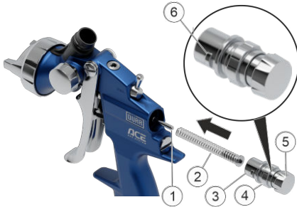
Fig. 13: Inserting the needle
