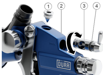
Fig. 17: Replace O-ring on the air control
