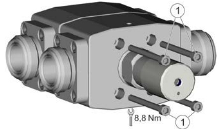
Fig. 24: Thread in the screws
