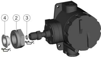
Fig. 20: Assemble pressure switch
