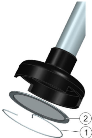
Fig. 30: Replace filter disk
