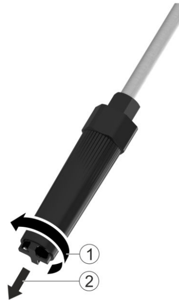
Fig. 31: Replace filter cartridge
