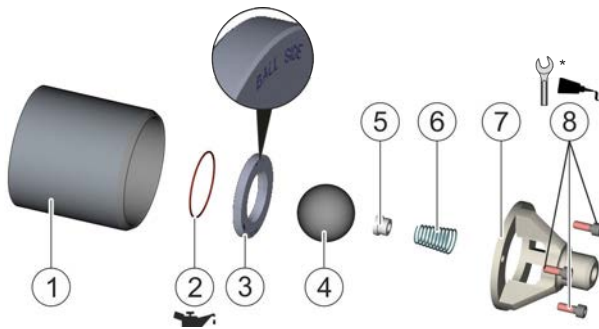
Fig. 19: Assemble non-return valve in the piston
