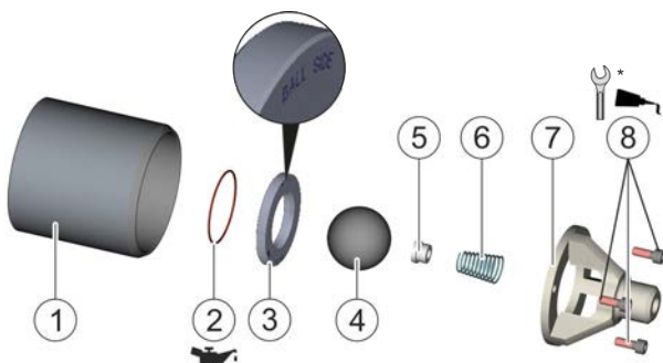
Fig. 22: Assemble non-return valve in the piston
