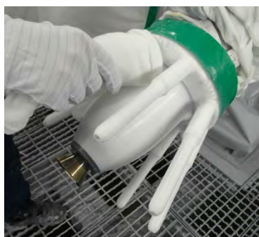
Fig. 38: Cleaning the electrode fingers
