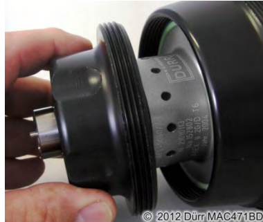
Fig. 66: Removing screw cap
