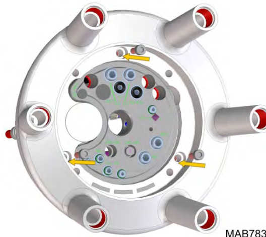
Fig. 25: Inserting the plastic screws
