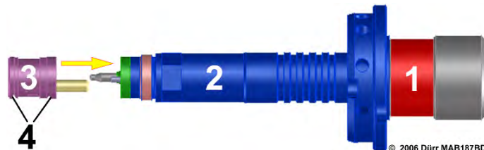
Fig. 88: Pushing up needle seat
