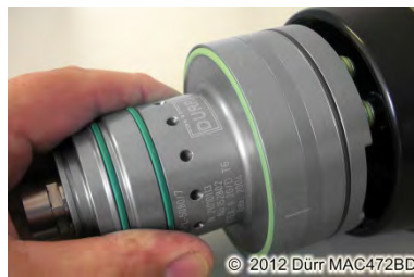
Fig. 67: Removing the turbine
