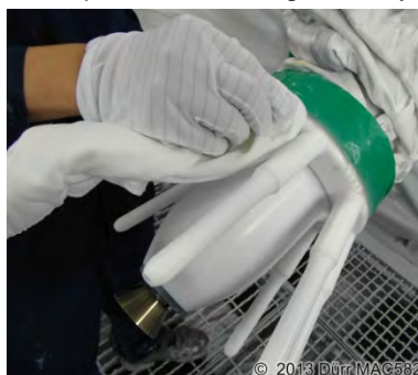
Fig. 39: Cleaning the electrode ring
