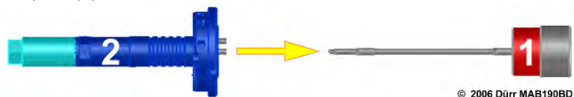
Fig. 91: Removing the assembly tool
