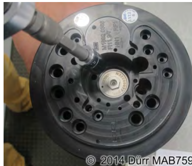
Fig. 80: Removing the main needle valve
