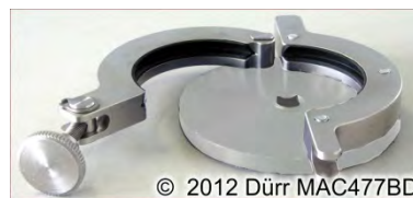
Fig. 45: Special tool for bell disk
