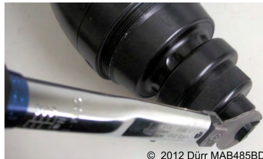
Fig. 70: Tightening the screw cap
