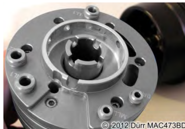
Fig. 68: Sealing rings at the turbine connections
