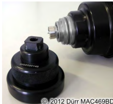
Fig. 64: Special tool for screw cap
