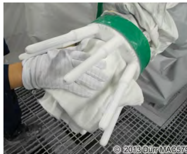
Fig. 36: Cleaning the atomizer body
