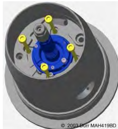
Fig. 172: Mounting bolts for the chuck
