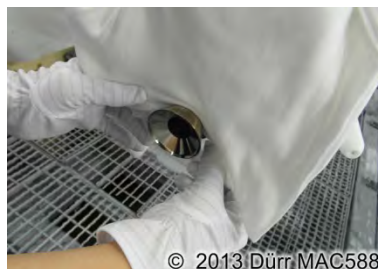
Fig.37: Cleaning the shaping air ring
