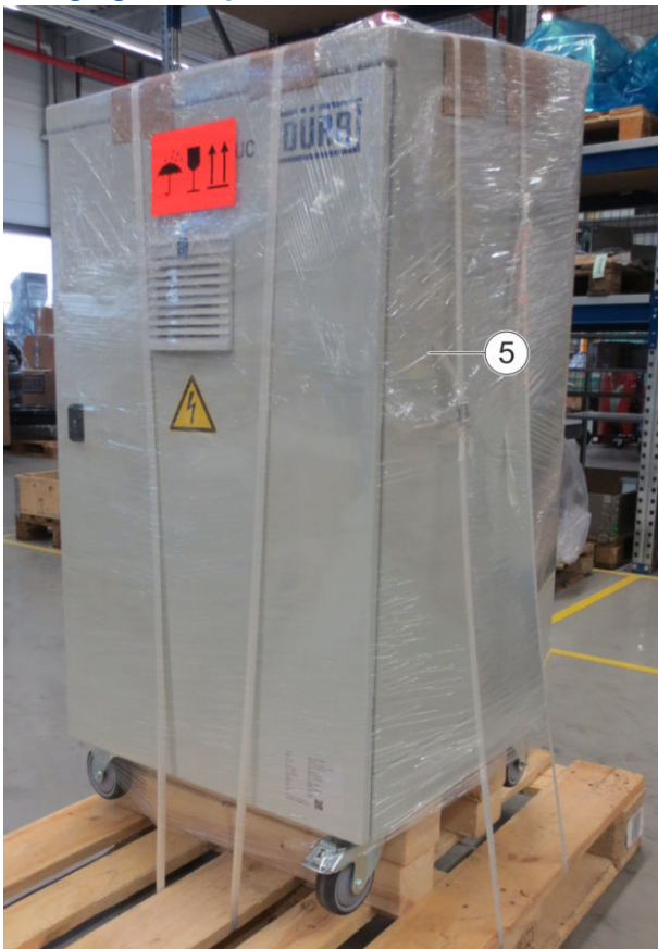
Fig. 14: Control cabinet wrapped in foil
