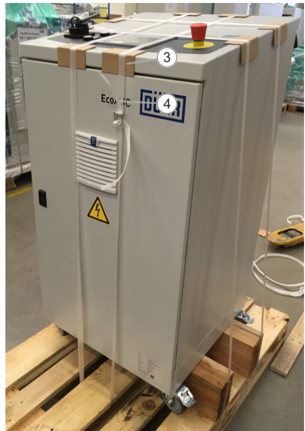
Fig. 13: Fixing Control cabinet
